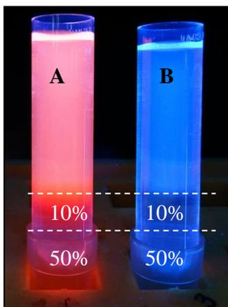
Fig. 5 QDs (A) and polymer (B) solutions after ultracentrifugation
