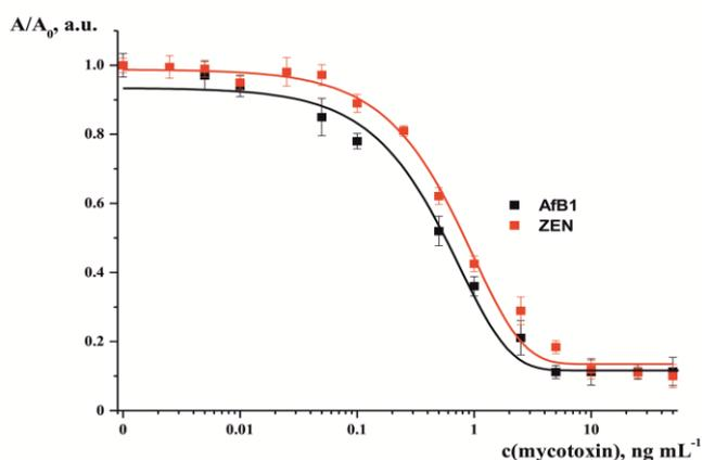
Fig. 8 Calibration curves for the mycotoxins determination by DAM FLISA.  $A/A_0$  is the relative luminescence ( $\lambda_{em} = 540$  nm for green QDs (ZEN determination), 594 nm for orange QDs (AfB1 determination)). Data indicate averages of fivefold determinations.
