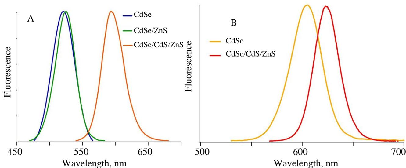
Fig. 2 Fluorescence spectra of CdSe core QDs and core-shell QDs:  $d(\text{CdSe}) = 2.3$  nm (A);  $d(\text{CdSe}) = 4.1$  nm (B). All spectra are normalized on peak maximum
