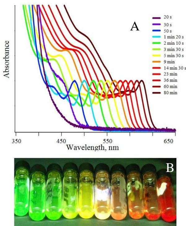
Fig. 1 The change of absorption spectra (A) and colour of fluorescence (B) of CdSe QDs during synthesis
