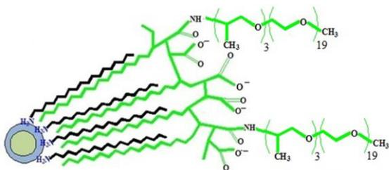
Fig. 4 The structure of hydrophilic QDs covered with the polymer
