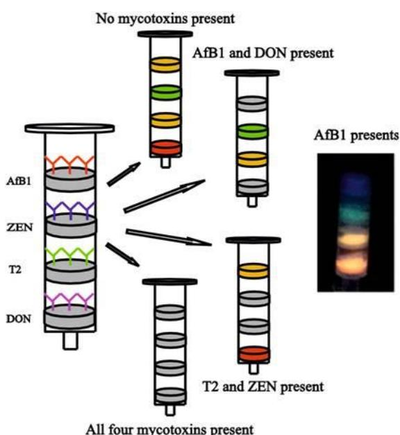
Fig. 9. Gel-based immunoassay set-up for simultaneous detection of deoxynivalenol, zearalenone, aflatoxin B1 and T2-toxin and examples of analysis outcomes
