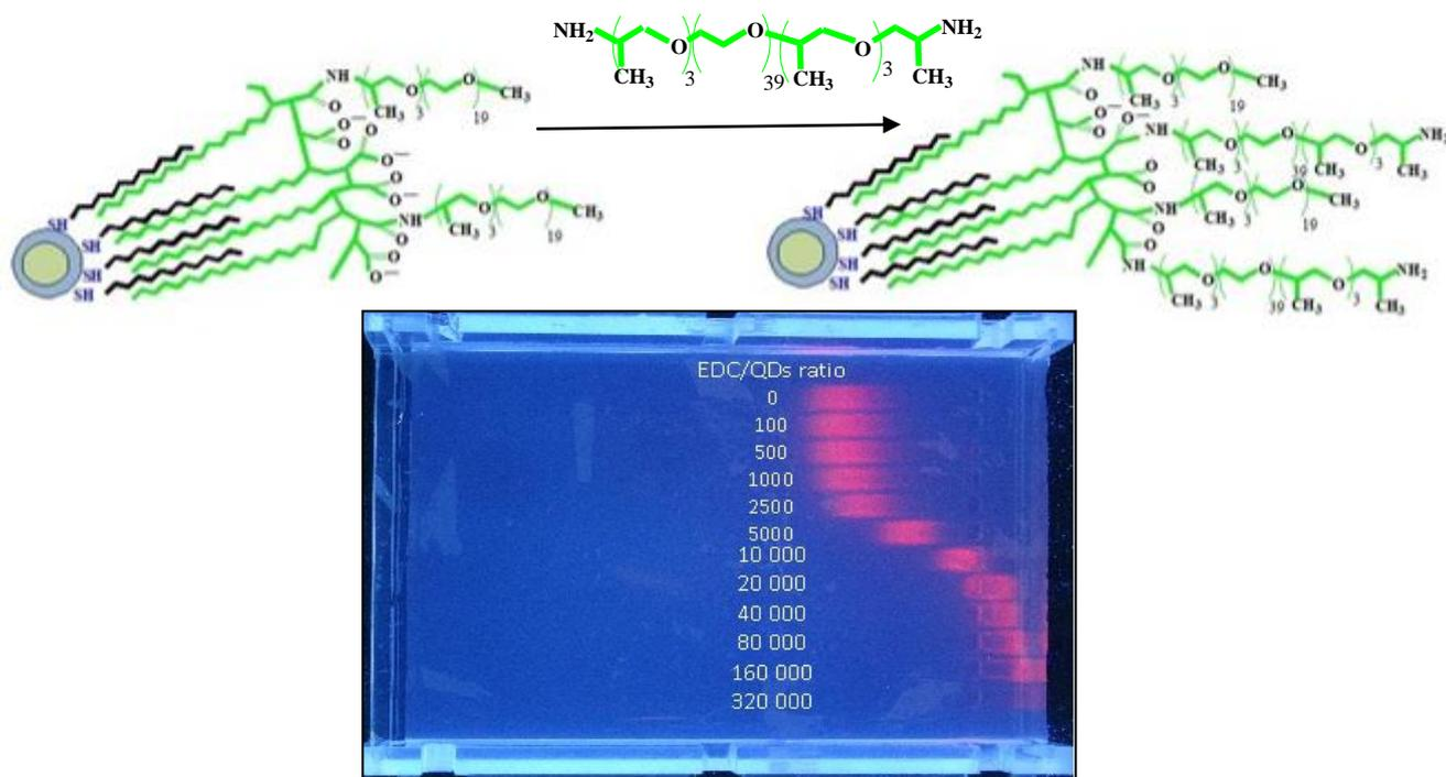
Fig. 6 Scheme of hydrophilic QDs interaction with Jeffamine ED 2003 and electrophoresis of the QDs produced with different amount of EDC
