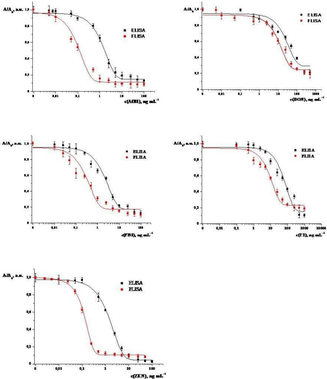
Fig. 7 Calibration curves for the mycotoxins determination by ELISA and FLISA.  $A/A_0$  is a relative analytical signal: absorbance ( $\lambda=450$  nm) for ELISA and luminescence ( $\lambda=540$  nm for green QDs, 594 nm for orange QDs and 642 nm for red QDs) for FLISA.
