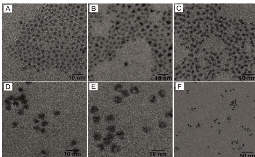
Fig. 3 TEM images: CdSe cores with fluorescence peak at 520nm (A) and corresponding core-shell QDs: CdSe/ZnS (B), CdSe/CdS/ZnS (C); CdSe cores with fluorescence peak at 605 nm (D) and corresponding core-shell CdSe/CdS/ZnS QDs (E) (all in toluene solution); hydrophilic CdSe/CdS/ZnS QDs ( $\lambda$ (em.)=594 nm) (F)
